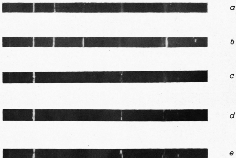
Fig. 10. Shows X-ray reflection from: (a) \text{Cu}_2\text{O} powder with small copper impurity. (b) \text{Cu}_2\text{O} film formed at 700^\circ\text{C} , 0.5 mm Hg air pressure and slowly cooled. (c) \text{Cu}_2\text{O} film formed at 900^\circ\text{C} at the same pressure and slowly cooled. (d) \text{Cu}_2\text{O} film formed at 1030^\circ\text{C} at the same pressure and slowly cooled. (e) \text{Cu}_2\text{O} film formed at 1030^\circ\text{C} at the same pressure but suddenly cooled.
