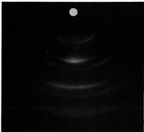
Fig. 5. Shows oriented rings of \text{Cu}_2\text{O} with 110 orientation. The rings strong at the centre are \sqrt{2} (near the shadow edge), \sqrt{8} and \sqrt{18} .
