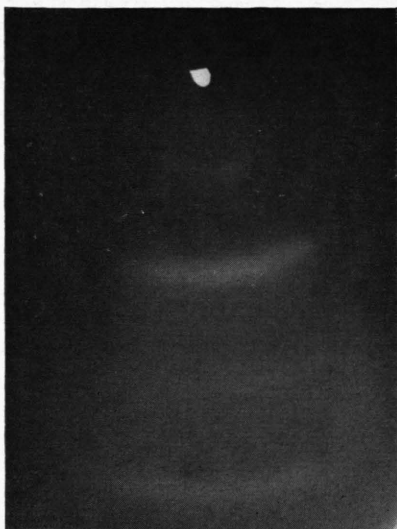
Fig. 9. Shows the four arc pattern, which approximately corresponds (vide Tab. 4) to 111, 222, 333 and 444 arcs of \text{Cu}_2\text{O} .
